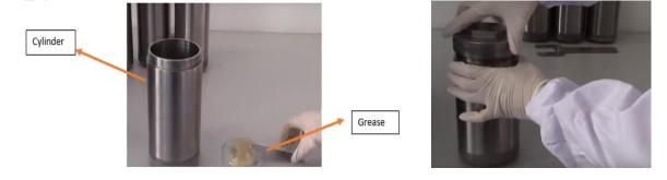
Figure 5: Grease with cylinder which have to be applied inside
