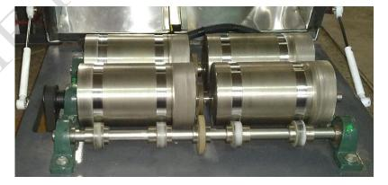
Figure 9: Roller for grease test
